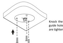
Knock the plastic rivets into the guide holes and ensure that they are tightened up.
